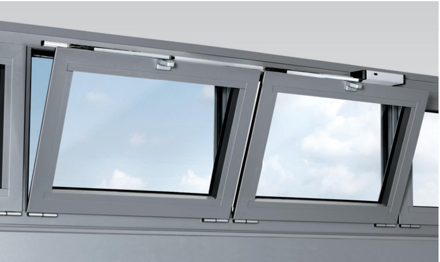
The fanlight opening system, consisting of the VENTUS fanlight opener and the ELTRAL electric drive, enables a cost-effective electromechanical control of several sash units. Due to the flat design of the opening stays, the system can be used for smoke exhaust and daily ventilation on inward opening, vertically installed square Bottom-Hung windows made of timber, PVC or metal with low space conditions.
