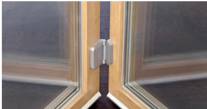
Height-adjustable sash hinge, view from outside; the screw connection is concealed from the outside which increases burglar inhibition
