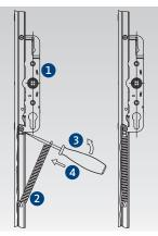
Installation of the tension spring for facilitated handle operation for sash weight > 200 kg  $\,$
