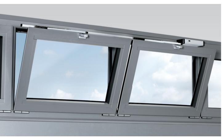
The fanlight opening system, consisting of the VENTUS fanlight opener and the ELTRAL electric drive, enables a cost-effective electromechanical control of several sash units. Due to the flat design of the opening stays, the system can be used for smoke exhaust and daily ventilation on inward opening, vertically installed square Bottom-Hung windows made of timber, PVC or metal with low space conditions.
