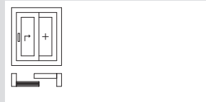
Pattern A 1 Lift&Slide door 1 Fixed-glazed sash Fig.: sliding direction to the right
