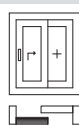
Pattern A 1 Lift&Slide door 1 Fixed-glazed sash Fig.: sliding direction to the right
