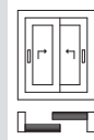
Pattern D 2 Lift&Slide doors Fig.: sliding direction to the right and left
