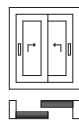
Pattern D 2 Lift&Slide doors Fig.: sliding direction to the right and left
