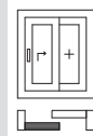
Pattern A 1 Lift&Slide door 1 Fixed-glazed sash Fig.: sliding direction to the right
