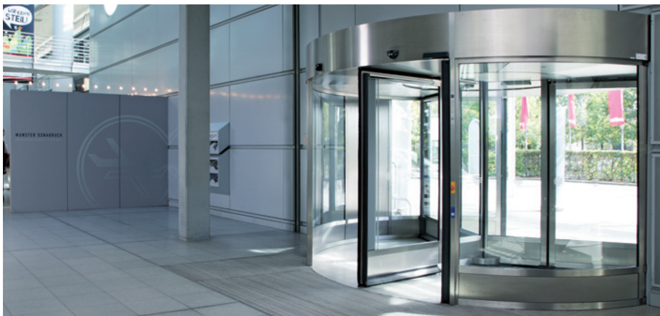
AIRPORT MÜNSTER-OSNABRÜCK | GREVEN | GGR large-capacity revolving door | fully automatic | 3-leaf | stainless steel panelling | leaf can be swung out for escape and rescue routes | \varnothing 4800 mm
