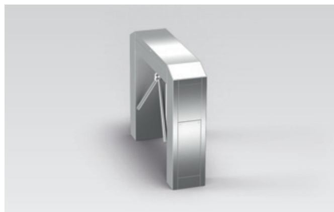
2-arm turnstile in release position: the turnstile underneath the housing turns when the doorman presses the button or when the alarm is triggered. The access or additional escape route is released. Normal operation can then be resumed quickly and easily at the push of a button.
