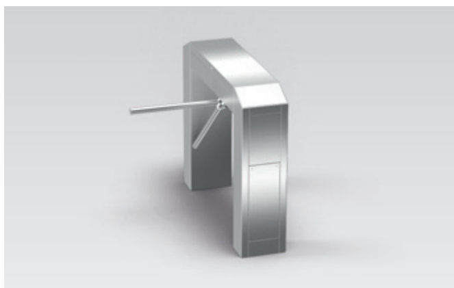
2-arm turnstile in normal operation: the electric brake holds the turnstile in the locked position. When a gentle pressure is applied, the drive is activated and turns the turnstile further through 120° or 240°.
