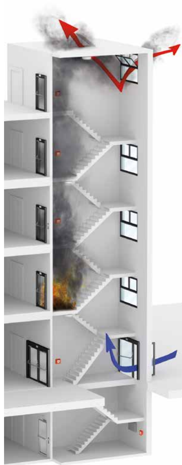
Schematic view of the functional principle of a smoke and heat exhaust ventilation system with supply air, skylight and facade opening
