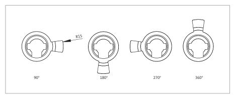
Other cam positions are required for special applications or for special lock types.
